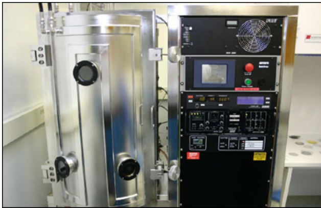
Figure 6.10 – Sputter Cu seed layer
