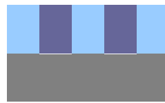
Figure 6.4 – PEB and Develop
