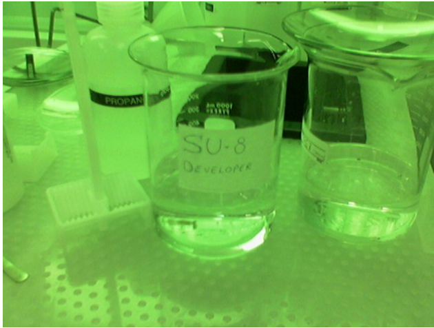
Figure 6.5 – Wet etching SU-8
