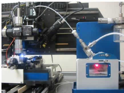
Aerosol-jet printing system used for 3D printing of graphene interconnects
