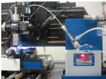
Aerosol-jet printing system used for
