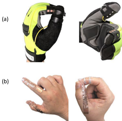
Figure 2. RFID Tip-Tap device (a) on a glove (b) as an on-skin tattoo
