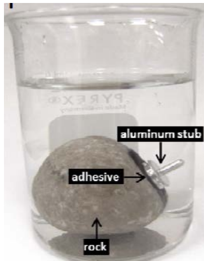
Bonding aluminum stub to a rock with bonding hydrogels in water
