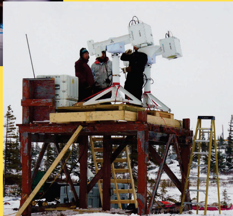
Dr. Claude Duguay and his team near Churchill, Manitoba, deploying and operating radar systems to advance remote-sensing research on snow.
