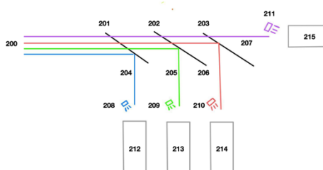
Fig. 3. Optical module with beam splitting mechanism for high efficiency utilization of full spectrum light sources
