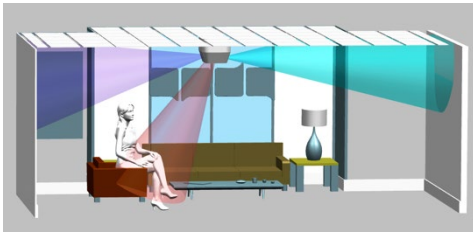
Fig. 1. Computer vision low energy directional lighting in an enclosed office space application
