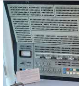
FIGURE 1: The diagnostic panel of the IBM System/360 Model 75, on display in the museum. It was installed at the University of Waterloo in 1967 and was thought to be the most powerful computer in Canada for a brief time.
