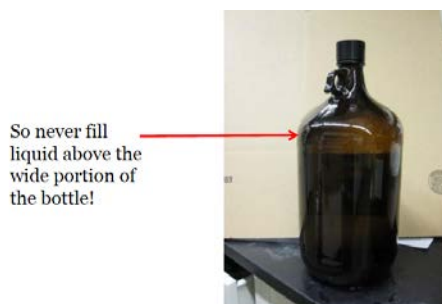
Figure 2: Example of the maximum fill level for liquids in a waste bottle.
