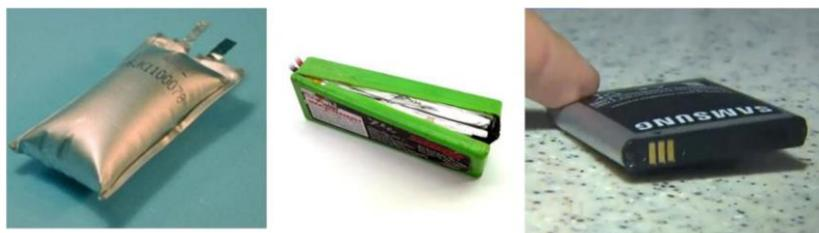
**Figure 5: Swollen lithium-ion pouch batteries**
