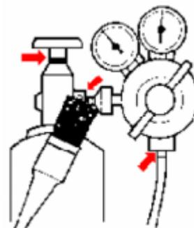
Figure 2: Schematic of a compressed gas cylinder components.
