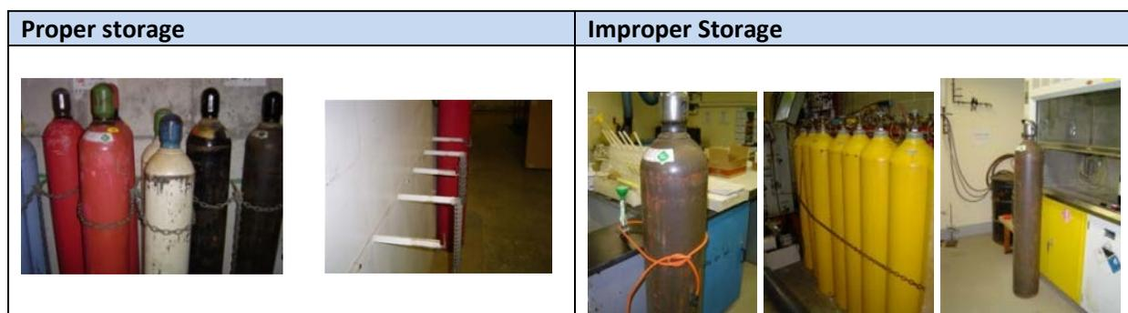
Figure 3: Differences between proper and improper storage.
