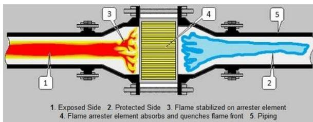
Figure 6: Schematic representation of how a flash arrestor works.
