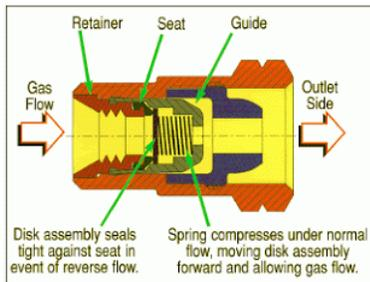
Figure 7: Schematic representation of how a check valve works.
