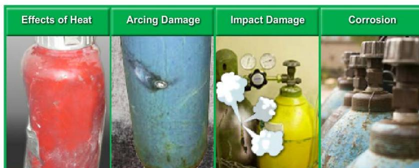
Figure 1: The four ways in which a compressed gas cylinder can be physically damaged.
