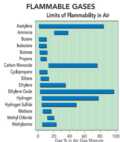
Figure 4: An illustration depicting the upper and lower flammability limits for various flammable gases.
