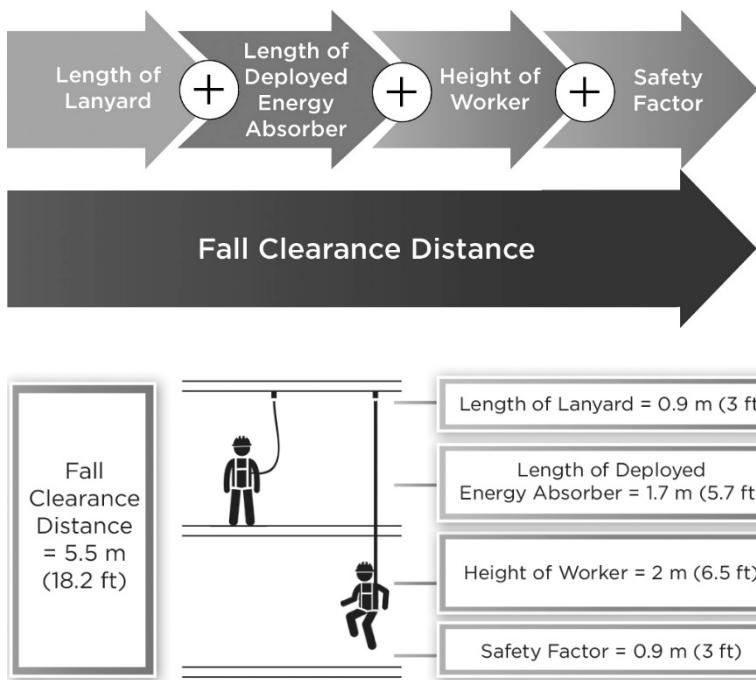
In this example, the worker's connection point to the anchor needs to be at least **5.5 m (18.2 ft)** from the ground or bottom level.
