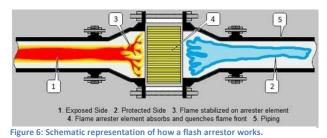
regulator. The arrestor consists of a series of small pathways or holes. As a flame travels through it this multitude of paths (or holes) the flame separates and its energy dissipates thus quenching the flame.
