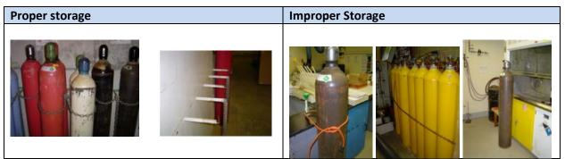
Figure 3: Differences between proper and improper storage.
