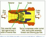
Figure 7: Schematic representation of how a check valve works.
