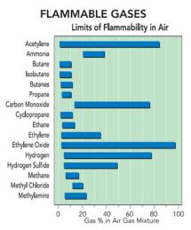
Figure 4: An illustration depicting the upper and lower flammability limits for various flammable gases.
