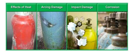
Figure 1: The four ways in which a compressed gas cylinder can be physically damaged.
