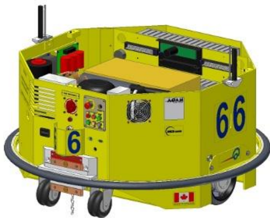
Fig4:ADAM allows companies to deliver the needed quantities of material, when and where they are needed—basic principles of lean manufacturing. But, even in 2012, many companies still use manual process for the transportation of raw and work-in-process material between an automated storage and retrieval system and an
