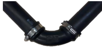
Figure 2. Flexible elbow coupling used to simulate socket welds
