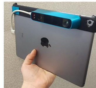
Figure 4. Structure IO, structured light scanner used for experiment mounted on an iPad
