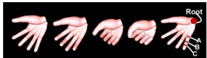
Fig. 3. Screen shots of an animated replicate of a hand movement used in this study. Local Euler angles were collected for the wrist (root) and three joints (A, B, and C) along each finger. Joints in each figure are named as shown on the little finger of the far right hand (e.g. in index finger, A: proximal joint, B: intermediate joint, C: distal joint).
