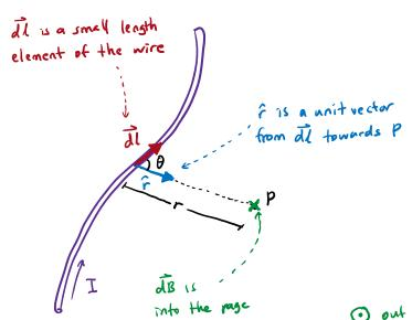
The differential magnetic field distance to the differential current element Idl 11:
