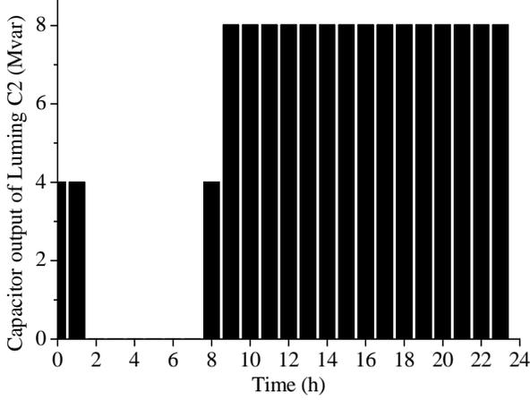
Fig.7. Optimal values of capacitor output obtained with the proposed algorithm for Luming C2 (MADSON = 8).
