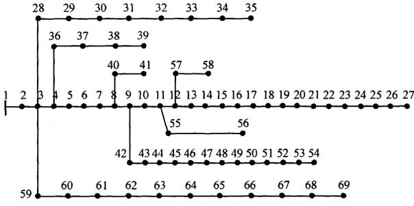
Fig.1. Schematic diagram of PG&E 69-bus system [18].
