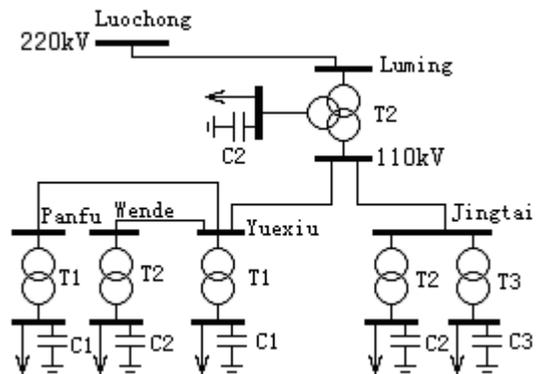
Fig. 6. Connection diagram of Luming 14-bus system.
