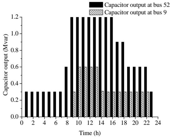
Fig.4. Optimal values obtained with the proposed algorithm for capacitor outputs for the 69-bus system (MADSON = 7).
