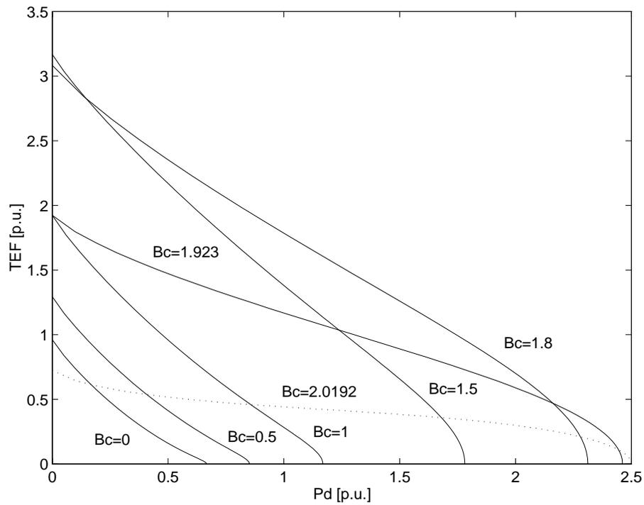
Fig. 10. Transient Energy Function profiles for the closest u.e.p. at different levels of shunt compensation  $B_C$  as  $\lambda = P_d$  changes. The system undergoes a Hopf bifurcation at  $B_C = 1.923$ .
