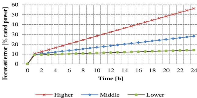
Fig. 5. Wind forecasting errors; and similarly for solar and demand powers
