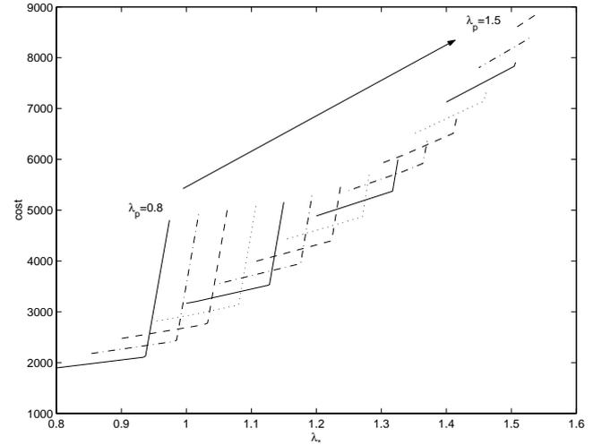
Fig. 7. Pareto-optimal set of values for the Linear Combination formulation applied to the 57-bus test system.
