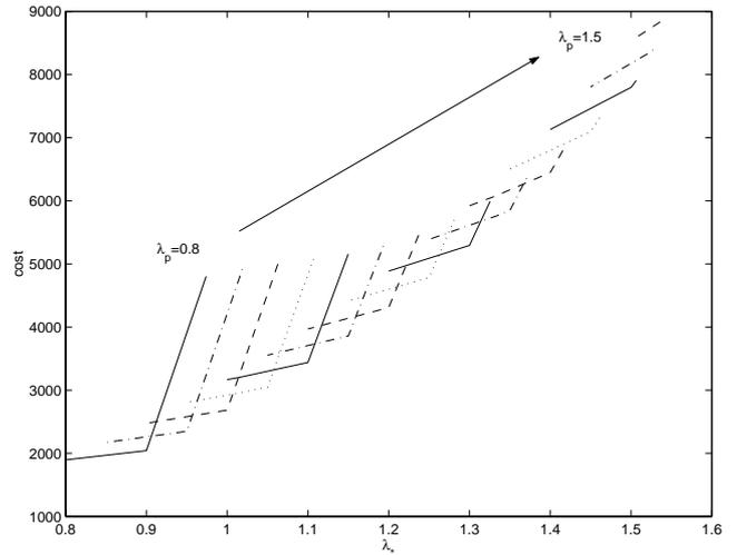
Fig. 14. Pareto-optimal set of solutions for the Goal Programming formulation considering reactive power costs ( $\omega_2 = 0.001$ ,  $\omega_3 = 1 - \omega_1$ ,  $\omega_4 = \omega_5 = 0.3$ ) applied to the 57-bus test system.
