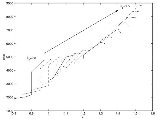
Fig. 11. Pareto-optimal set of solutions for the Goal Programming formulation ( $\omega_2 = 0.001$ ,  $\omega_3 = 1 - \omega_1$ ) applied to the 57-bus test system.
