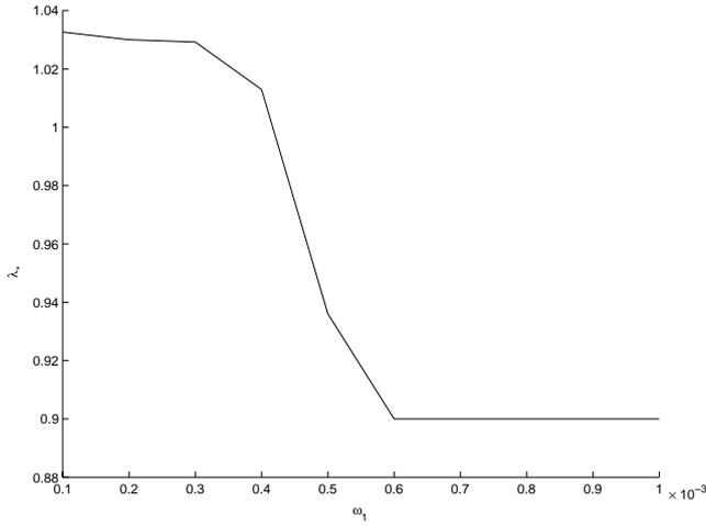
Fig. 4. Maximum loading versus weighting factor  $\omega_1$  for the Linear Combination formulation applied to the 57-bus test system for  $\lambda_p = 0.9$ .
