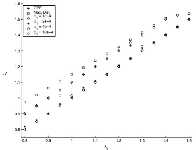
Fig. 10. Maximum loading point versus current operating point for the Goal Programming ( $\omega_2 = 0.001$ ,  $\omega_3 = 1 - \omega_1$ ) and Maximum Loading Distance formulations for the 57-bus test system.
