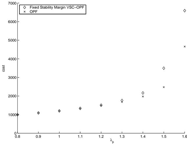
Fig. 8. Cost versus current operating point for the Fixed Loading Margin and traditional OPF formulations for the 118-bus test system.
