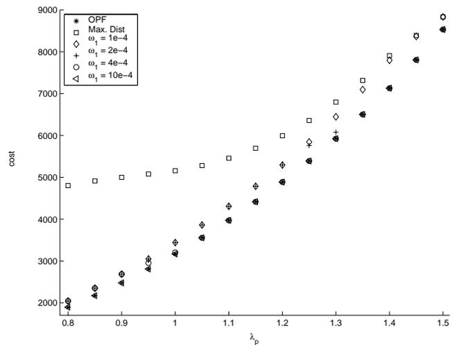
Fig. 9. Cost versus current operating point for the Goal Programming ( $\omega_2 = 0.001$ ,  $\omega_3 = 1 - \omega_1$ ), Maximum Loading Distance and traditional OPF formulations for the 57-bus test system.
