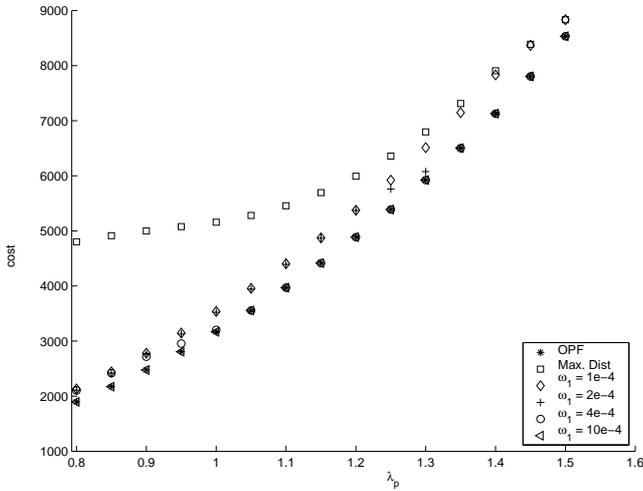
Fig. 5. Operating costs versus current operating point for the Linear Combination formulation, Maximum Loading Distance and traditional OPF for the 57-bus test system.
