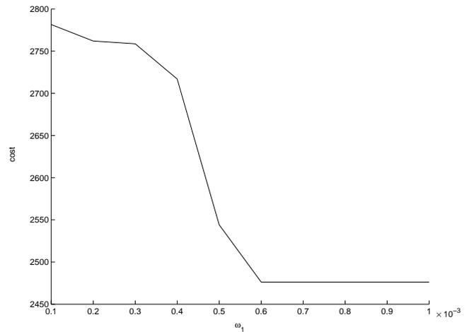
Fig. 3. Operating costs versus weighting factor  $\omega_1$  for the Linear Combination formulation applied to the 57-bus test system for  $\lambda_p = 0.9$ .
