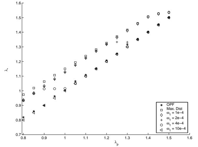
Fig. 6. Maximum loading point versus current operating point for the Linear Combination and Maximum Loading Distance formulations for the 57-bus test system.
