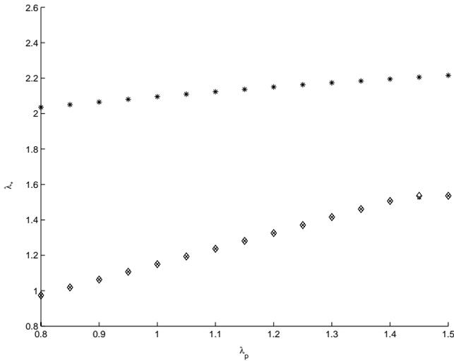
Fig. 1. Maximum loading versus current operating point using the Maximum Loading Distance problem for the 57-bus test system. The symbols \*,  $\diamond$ , and  $\times$  correspond to solutions for the system with no limits, generator P and Q limits, and both bus voltage limits and generator P and Q limits, respectively, at the maximum loading point; operating limits are always enforced at the current operating point.
