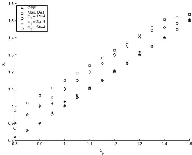
Fig. 13. Maximum loading point versus current operating point for Goal Programming formulation considering reactive power costs ( $\omega_2 = 0.001$ ,  $\omega_3 = 1 - \omega_1$ ,  $\omega_4 = \omega_5 = 0.3$ ) and Maximum Loading Distance formulations for the 57-bus test system.
