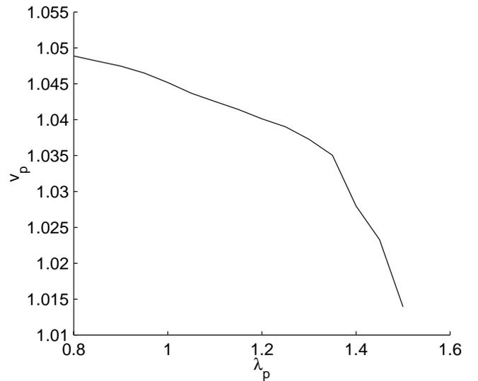
Fig. 2. Change in voltage magnitude at Bus 30 versus  $\lambda_p$  for the 57-bus test system.
