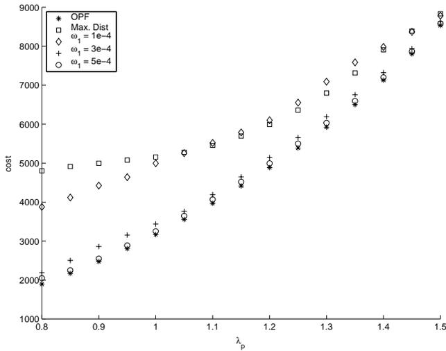
Fig. 12. Cost versus current operating point for the Goal Programming formulation considering reactive power costs ( $\omega_2 = 0.001$ ,  $\omega_3 = 1 - \omega_1$ ,  $\omega_4 = \omega_5 = 0.3$ ), Maximum Loading Distance and traditional OPF formulation for the 57-bus test system.
