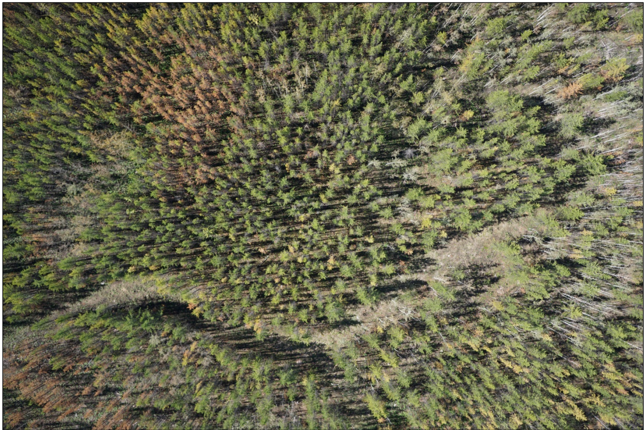
Figure 17: Example of high relief displacement with trees leaning away from the center of the image. Data from Fraser et al. (2015).
