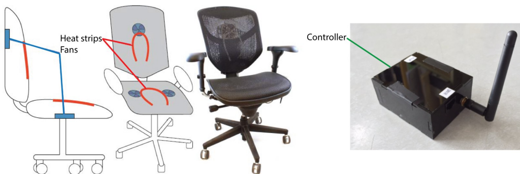
Figure 1. PCS chair developed by the Center for the Built Environment at the University of California, Berkeley. The images show hardware and heating and cooling elements of the chair and the new controller with wireless connectivity.
