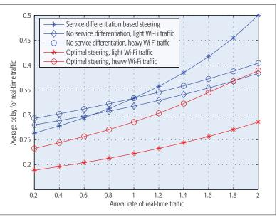
FIGURE 5. Delay performance through traffic steering.
