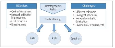
FIGURE 2. Traffic steering in LTE with unlicensed bands.
