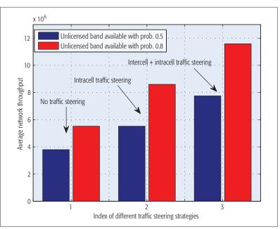
FIGURE 4. Aggregate throughput through traffic steering.
