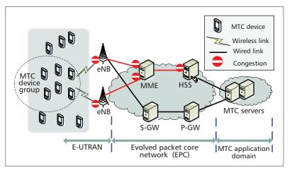
Figure 2. Authentication signalling congestion
