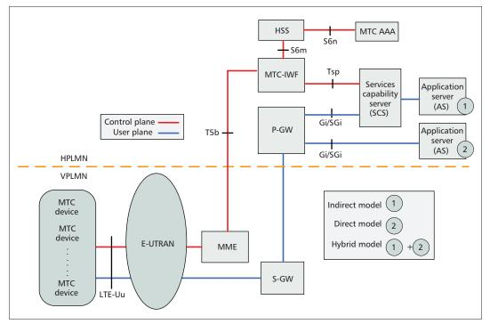
Figure 1. 3GPP security architecture for MTC.
