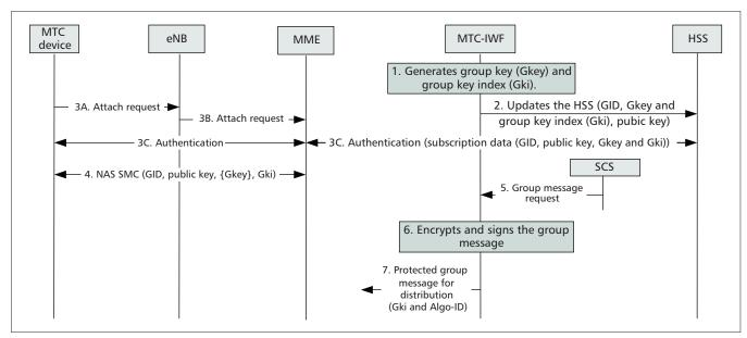
Figure 4. Network based protection for cell broadcast.
