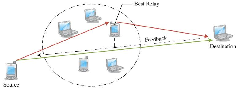
Figure 1. Amplify-and-forward opportunistic relaying with adaptive transmission.
