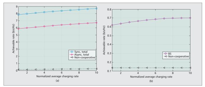
Figure 4. Rate comparison under various charging rate: a) total power constraint; b) BS power constraint.
