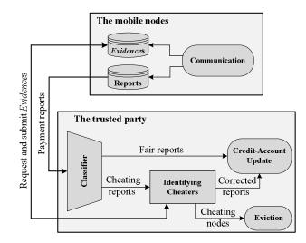
Fig. 2: The architecture of RACE.
