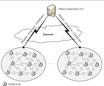
Fig. 1: The architecture of the considered network.
