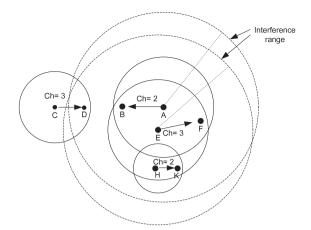
Figure 2. The asymmetrical transmission power can occur without control over multiple channels.
