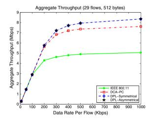
Figure 7. Aggregate throughput in the chain topology with different network loads.
