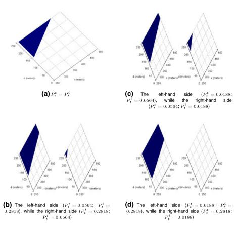
Figure 3. The effect of using different transmission power over a channel. The shadowed areas are the vulnerable areas where collisions occur.
