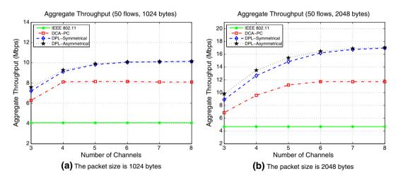
Figure 11. Aggregate throughput versus number of channels in the random topology.
