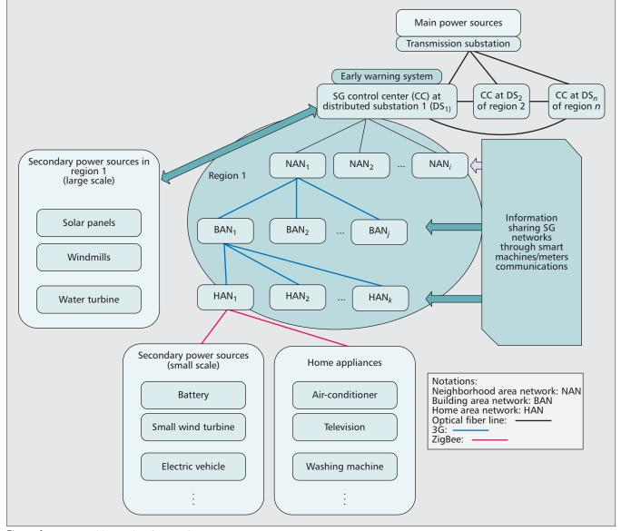
Figure 1. Smart grid hierarchical networks.
