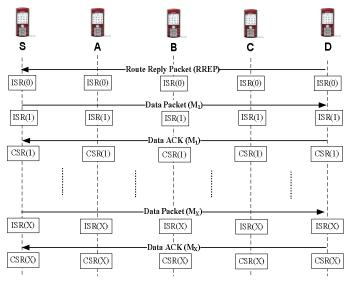
Fig. 5: The composed receipts when the last packet is data, ACK or RREP.
