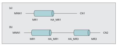
Figure 2. Examples of tunneling in NEMO BS: a) MNN1 communicates with CN1; b) MNN1 communicates with CN2.
