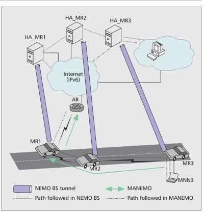
Figure 4. Optimization of routes to reach the CN in multi-hop communications.
