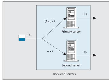
Figure 4. The deployment of primary and second servers to achieve reliability.
