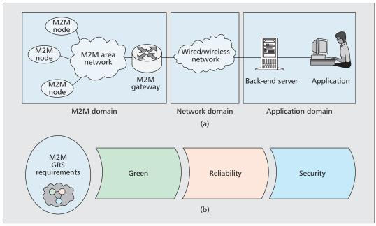
Figure 2. M2M communications: a) architecture; b) GRS requirements.
