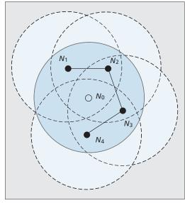
Figure 3. An example that node  $N_0$  may switch to sleep mode because its sensing range is fully covered by the connected neighbors  $N_1, ..., N_4$ .
