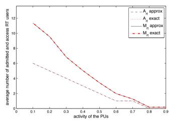
Fig. 9. Approximated and exact number of admitted RT users,  $A_{rt}$ , and access RT users,  $\overline{M}_{rt}$ , for different values of the activity of the PUs,  $\delta$ ; for N = 20 channels,  $P_D = 0.01$ ,  $P_B = 0.1$ , and l = 20 packets.
