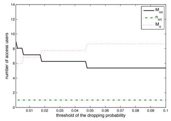
Fig. 12. Average number of the RT access users,  $\overline{M}_{rt}$ , NRT access users,  $\overline{M}_{nrt}$ , and NRT allocated channels,  $\overline{n}_{nrt}$ , for different threshold values of the dropping probability,  $P_D$ ; for N = 20 channels,  $\delta = 0.3$ ,  $P_B = 0.1$ , and l = 20 packets.
