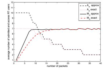
Approximated and exact number of admitted RT users, Art, and Fig. 6. access RT users,  $\overline{M}_{rt}$ , for different number of packets, l, when N = 20channels,  $\delta = 0.3$ ,  $P_D = 0.01$ , and  $P_B = 0.1$ .
