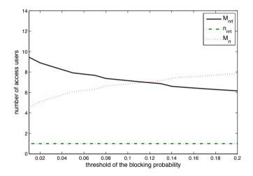
Fig. 13. Average number of the RT access users,  $\overline{M}_{rt}$ , NRT access users,  $\overline{M}_{nrt}$ , and NRT allocated channels,  $\overline{n}_{nrt}$ , for different threshold values of the blocking probability,  $P_B$ ; for N = 20 channels,  $\delta = 0.3$ ,  $P_D = 0.01$ , and l = 20 packets.
