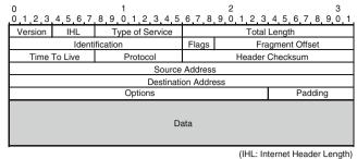
Fig. 3 Data packet format
