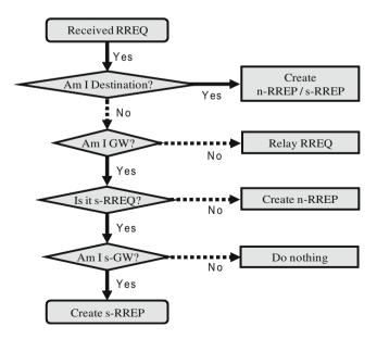
Fig. 5 Algorithm of the response to received RREQ
