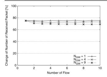
Fig. 8 Degradation of number of received packet: comparison between the experiment with background traffic and the one without
