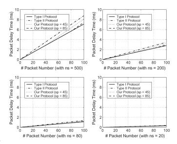
Fig. 6. Relation between the packet delay time and the packet number  $n_p$ .
