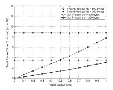
Fig. 7. Relation between the total packet time cost and the valid packet ratio  $\rho_i$ .
