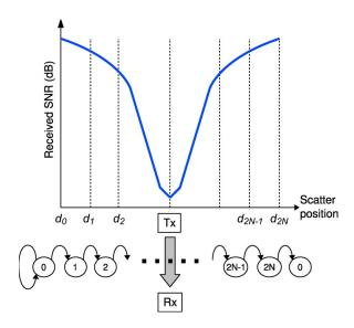
Fig. 2. Partition method for the Markov channel model with a single scatter.
