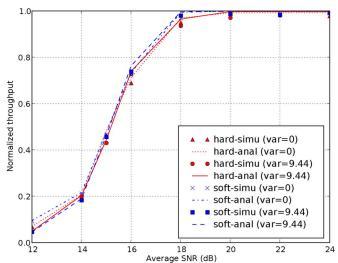
Fig. 5. Normalized throughput of the DRP versus the average SNR with different reservation methods, for  $\alpha=0.5$  and S=7, and the vacation periods follow (23) with the same mean  $\overline{V}=4$  but different variances.
