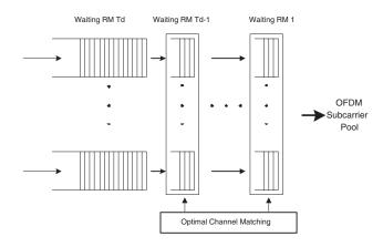
Fig. 3. Prioritized assignment based on packet delay.
