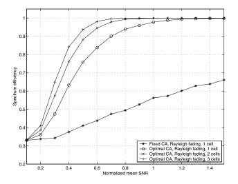
Fig. 4. Comparison of optimal assignment vs fixed assignment.
