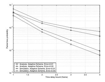
Fig. 9. Packet loss probability for the ADP scheme.
