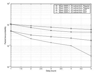
Fig. 7. Comparison of packet loss probability for the regular and EDT schemes.
