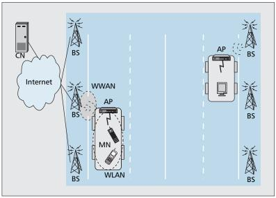
**Figure 1.** *Mobile hotspot architecture.*
