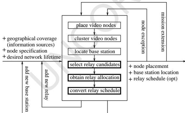
Fig. 9. Topology control iterations for wireless sensor networks.
