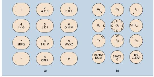
Figure 2. Keypad layouts: a) Less-Tap; b) MessagEase.
