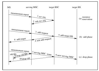
Figure 2: Soft handoff signalling.
