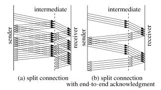
Fig. 8. Split connection with/without end-to-end acknowledgment.
