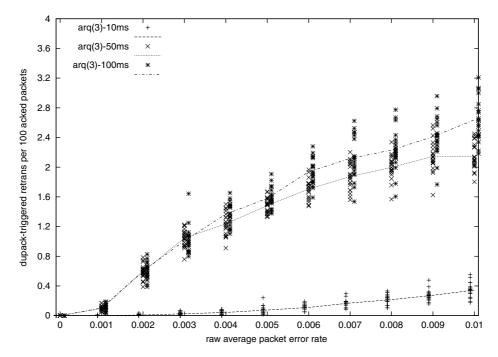
Figure 10. Dupacks with various wireless delays.
