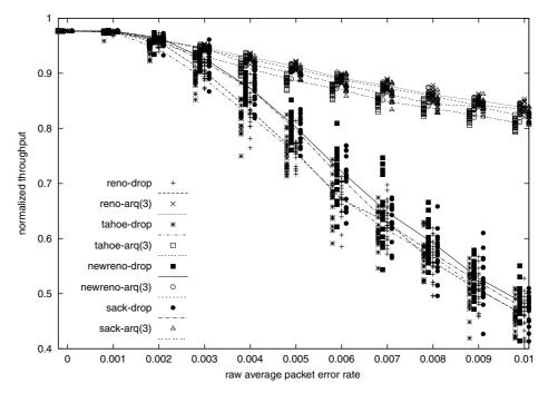
Figure 3. Normalized throughput for various TCP variants.
