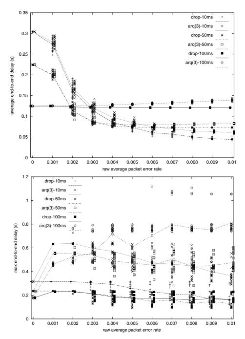
Figure 6. Average and maximum packet delay with various wireless delays.
