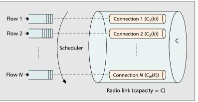
**Figure 4.** A queuing model of the CDGPS scheme.
