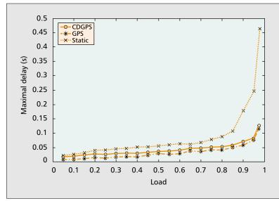
Figure 6. *Maximal delay comparison*.
