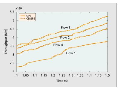
Figure 8. Throughput comparison of CDGPS and GPS (different weights).
