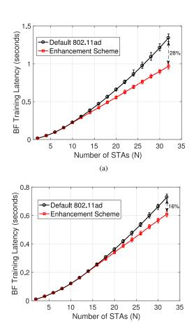
Fig. 10. Average BF training latency comparison in terms of different system parameters. (a) M = 8. (b) M = 12.
