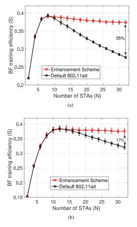
Fig. 9. BF training efficiency comparison in terms of different system parameters. (a) M = 8. (b) M = 12.
