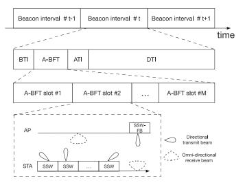
Fig. 1. The 802.11ad beacon interval format and an illustration of BF training procedure.
