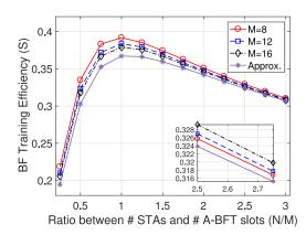
Fig. 8. BF training efficiency with respect to different ratios of the number of STAs to the number of A-BFT slots.
