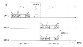
Fig. 2. Illustration of the BF training protocol. The BF training in A-BFT slots #1 is successful, while that in A-BFT slot #2 is unsuccessful since this A-BFT slot is selected by two STAs simultaneously.
