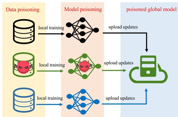
Fig. 14. Illustration of data poisoning and model poisoning.
