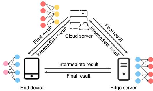
Fig. 12. Illustration for model partitioning in EECC.
