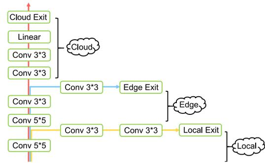
Fig. 13. Illustration for model early exiting in EECC.
