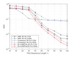
Fig. 10. SER performance versus pilot sequence length L with different lengths of transmitted messages J.
