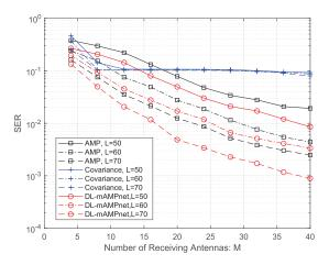
Fig. 9. SER performance versus number of receiving antennas M for J=1 bit.
