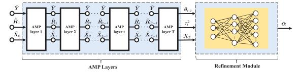
Fig. 3. Network architecture of the proposed DL-mAMPnet.
