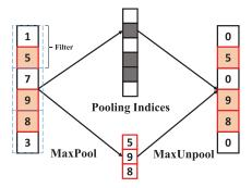
Fig. 6. Illustration of the MaxPool-MaxUnpool process.
