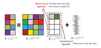
Fig. 2. Pictorial representation of the signal model.
