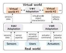
Fig. 3. The architecture of ISO/IEC 23005 (MPEG-V) standards [23].  $R \rightarrow V$  adaptation means the conversion of sensory data from the real world (RW) to virtual world (VW) object characteristics.  $V \rightarrow R$  adaptation means the conversion of sensory effects from VW into actuator commands to RW.  $V \rightarrow V$  adaptation means the conversion of native representations of information in a VW to the standard format.
