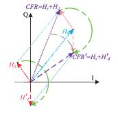
Fig. 2. Impact of the  $H_d$  phase on the overall CFR power.
