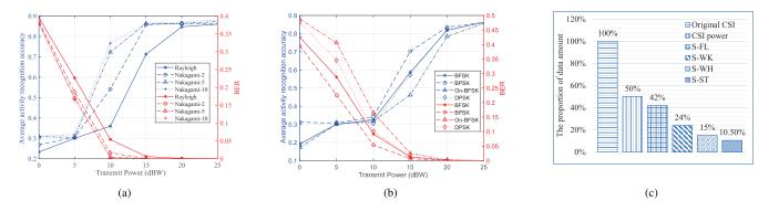
Fig. 10. Impact of wireless transmission on recognition accuracy and the data amount comparison before and after semantic encoding.
